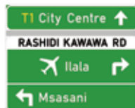
GD1 Direction Sign (in advance of a junction) with one cross street name
