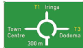
GD8 Direction Sign (in advance of a roundabout)
